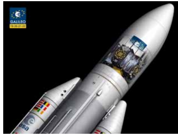
Vier FOC Navigationssatelliten an Bord einer Ariane 5 ES ©ESA/ P. Carril Four FOC navigation satellites accommodated on an Ariane 5 ES launcher
